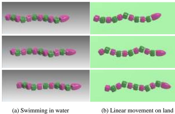
Fig. 7 Snapshots of amphibious locomotion with 11 modules employed with covers, using control parameters  $A=45.0$ ,  $T=1.0$ ,  $\varphi=2.1$  and  $O=0.0$ .
