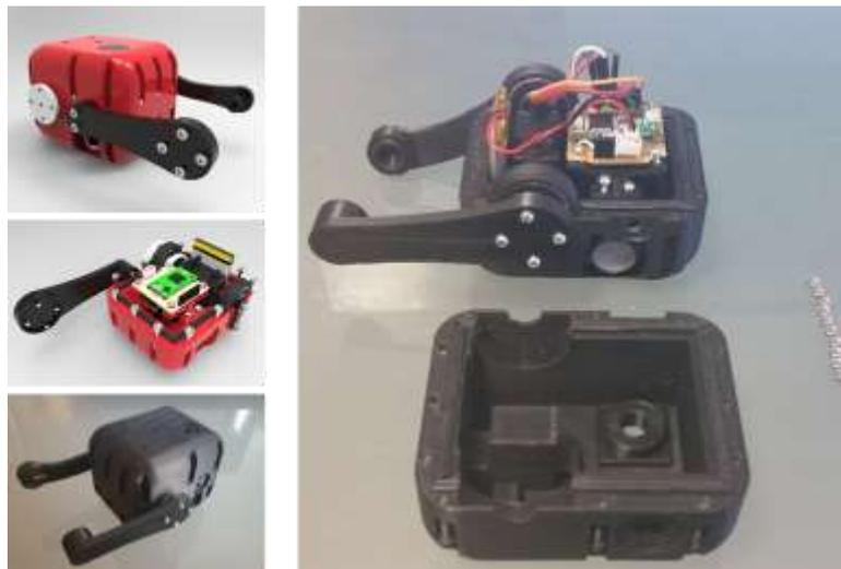
Fig. 3. Final design and 3D printed module
