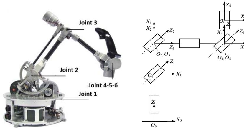
**Fig. 1.** The NHD prototype and its kinematic coordinates based on the DH method
