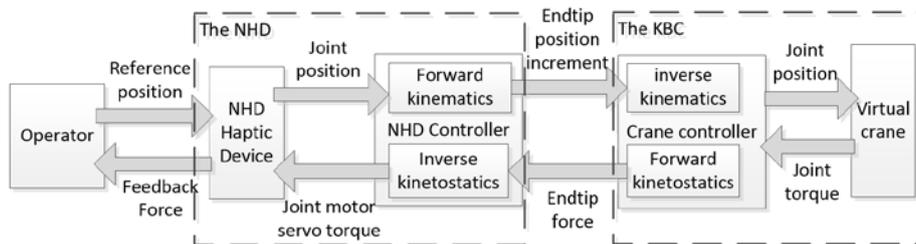
**Fig. 3.** The control architecture of the virtual crane simulator with force feedback
