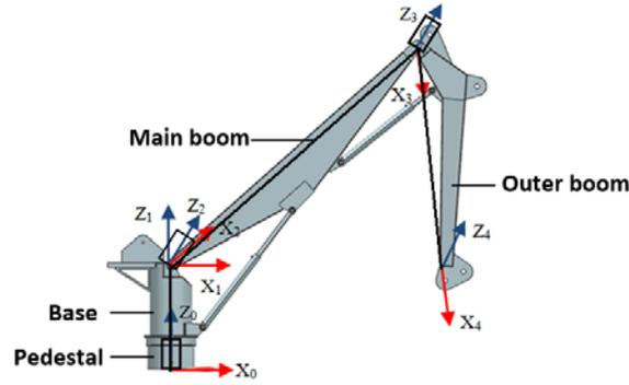
Fig. 2. The KBC and its kinematic coordinates based on DH method
