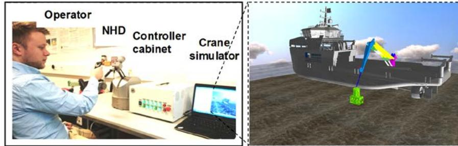
Fig. 5. The virtual marine crane simulator with force feedback
